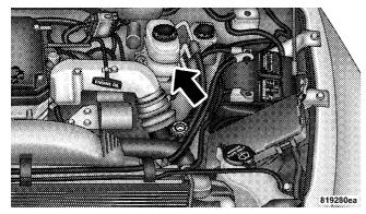
The brake master cylinder has a translucent plastic reservoir. On the outboard side of the reservoir there is a
